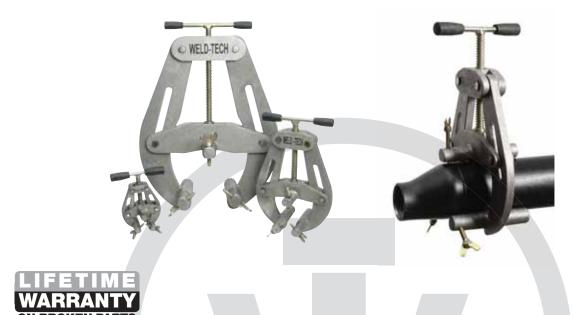
Due to its unique design, WT Clamp ensures that the clamping forces are evenly spread round the pipe to be welded, because the distance between clamping points are exactly the same. This is true for all pipe dimensions within the range of the WT Clamp (1 to 14 inches).
